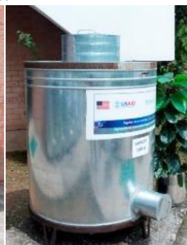
Figure 10 a metal silo with 1 ton storage capacity
