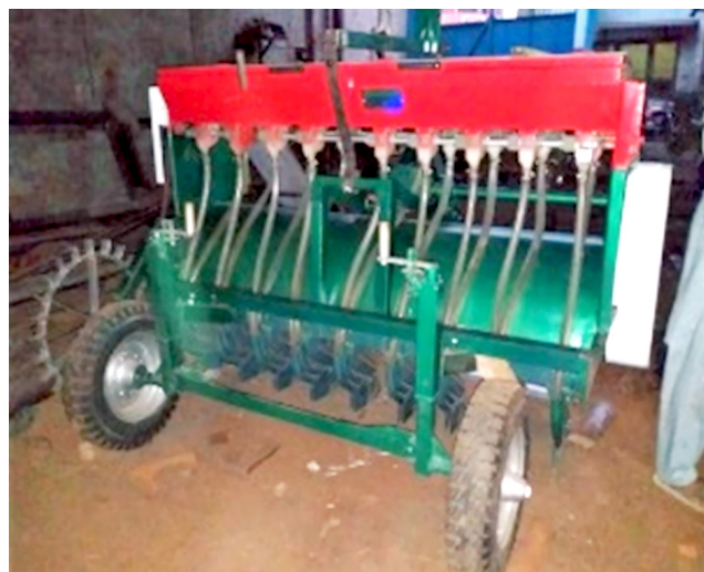
ZTHS with wheels manufactured by Sharif Engineering, Faisalabad.
