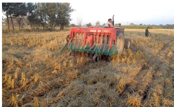
Pilot testing of the locally manufactured ZT Happy Seeder in a farmer's field in Punjab Province, Pakistan.
