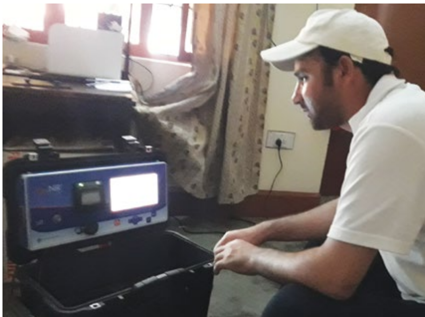
Using AgriNIR to analyse maize silage samples.
