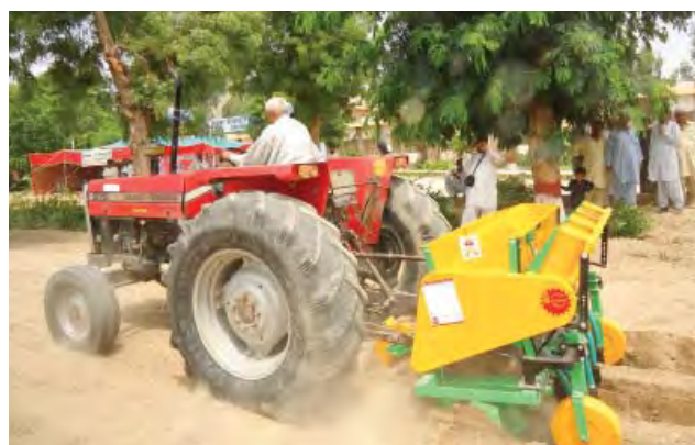
Field Day multi-crop bed planter - pilot testing.
